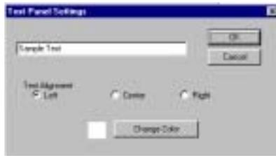
A Text gauge is another very simple gauge. It allows you to place a bit of text on the screen - just one line at a time. This is a convenient way to place a reminder on the screen such as "Max Temp 225°".
