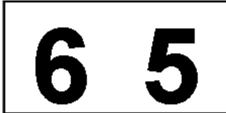
This is one of the simplest gauges. You may choose to show either or both the Gear Selected and the Gear Attained. The Gear Selected will show "6" when you put it into "Drive", but it will automatically change when the engine brake is activated or if you press the Down or Up arrows on the shift console. The Gear Attained shows the gear the transmission is actually in.
